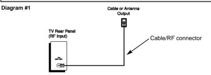
1) Connect an RF Cable from the wall outlet into the RF Cable In on the back of the TV.
